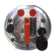
YSI buoys are made with marine-rated materials for years of operation. Above: Pressure cases made with non-corrosive materials and submersible connectors.
