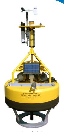
The scalable buoy can accommodate multiple instruments.
