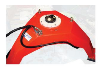
SonTek, a YSI subsidiary, offers a variety of current and wave monitoring options. Above: An economical set-up for monitoring current and waves from the sea floor. This solution is cabled to the surface.
